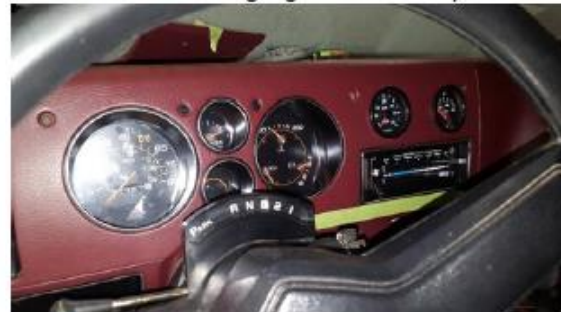
In need of tachometer and transmission temp gauge so drilled the dash for the new gauges. A little scary but turned out fine.
