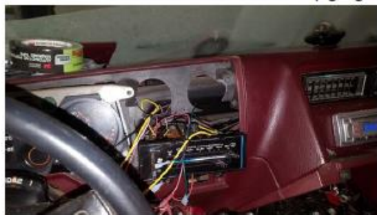
In need of tachometer and transmission temp gauge so drilled the dash for the new gauges. A little scary but turned out fine.
