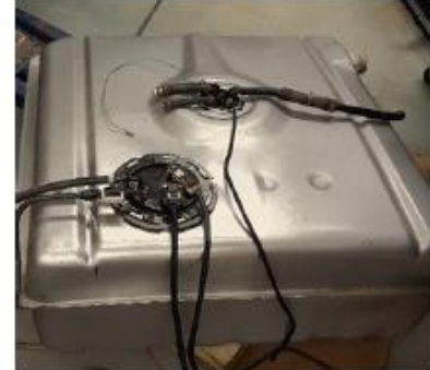
Modified new gas tank, added fuel pump system from donor for computerized pump control, left old sending unit and vent.
