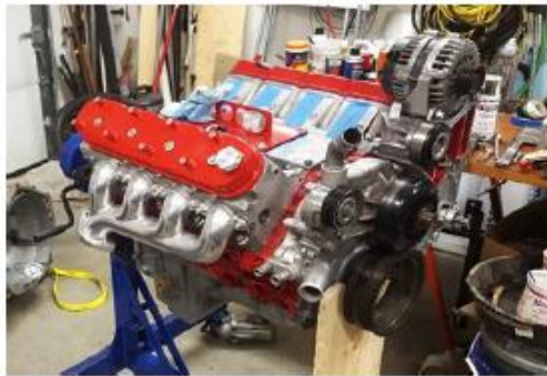
Cleaned up, new seals, timing gears and chain and ready for install.
