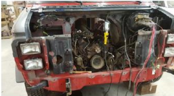
Cleaned bay of rust proofing, re-painted, installed new motor mounts and adapters.
