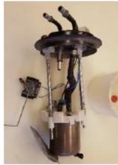
Modified new gas tank, added fuel pump system from donor for computerized pump control, left old sending unit and vent.
