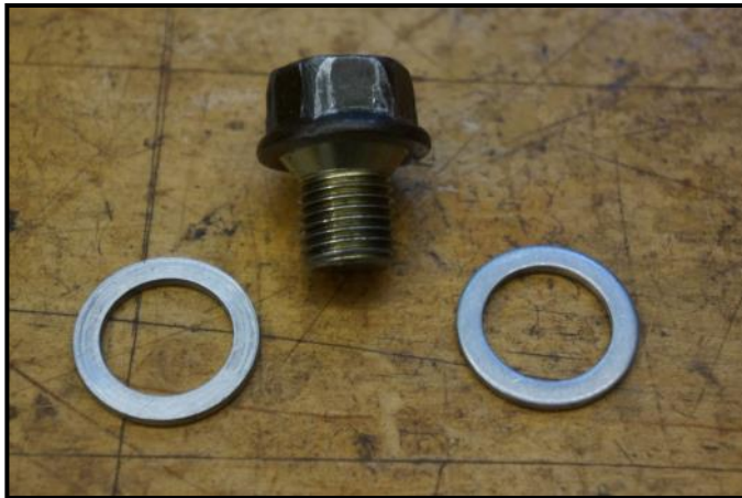
Used washer (L) shows crush marks. New one (R) will do better job, costs pennies
