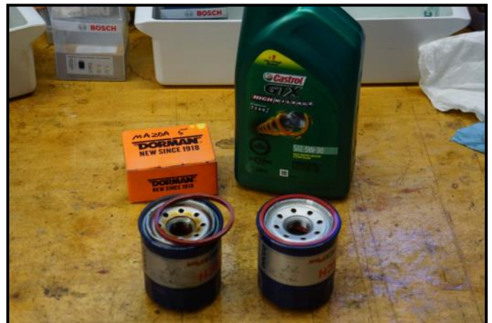
Old filter (L) has loose gasket. Add light coat of oil to new gasket. Orange box holds drain plug washer supply
