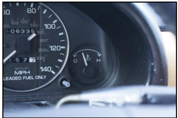
Get the temp gauge to move off "C" before draining the oil.
