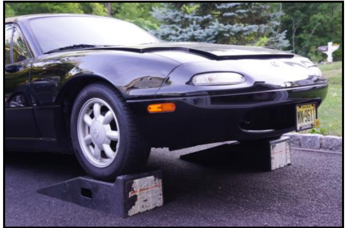
When using ramps, also use the parking brake. Chocks on the rear wheels are a good idea too.
