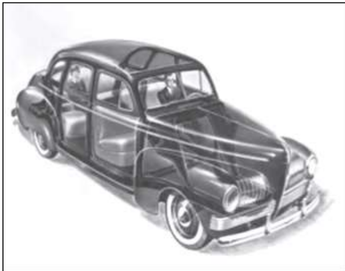
The 1941 Nash 600 pioneered the fully integrated monocoque body type with stressed skins—the first American car to use this modern architecture
