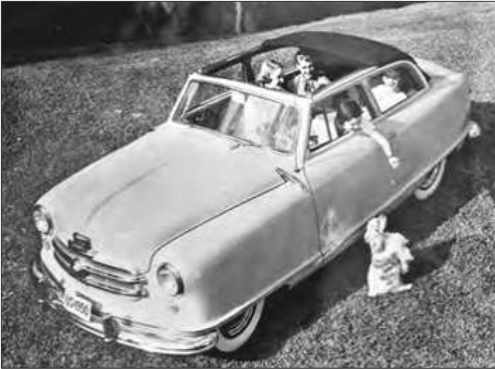
The Rambler, introduced in March 1950, became America's first postwar compact. Offered as convertible or wagon, its 82-hp Six delivered 30 mpg
