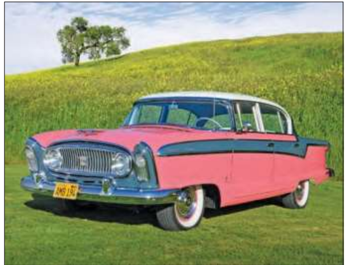
By 1956, full-sized Nashes shared bodies with Hudson. Both offered Packard-sourced V8s and General Motors Hydra-Matic transmissions
