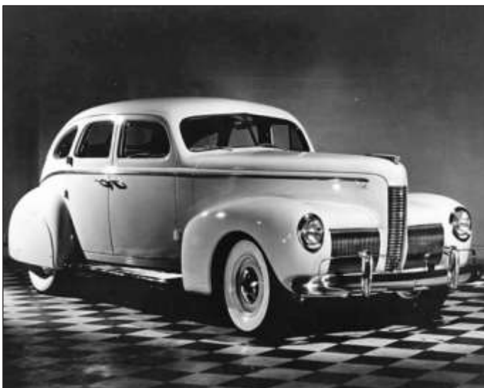
Top-of-the-line Nash Ambassador Eight for 1940 cost $1195. It had an overhead -valve straight eight that developed 115 horsepower.
