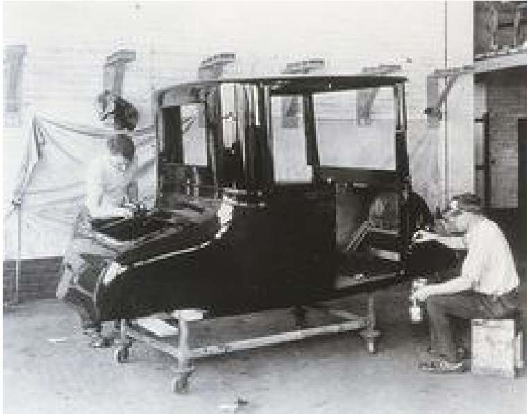
Above: Workers painstakingly apply varnish at a Fisher Body plant around 1915. Despite their intricate hand labor, it would start to peel and fade within a year.
