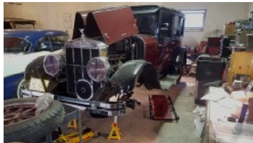
Found bad king pin bushings on inspection this year.
