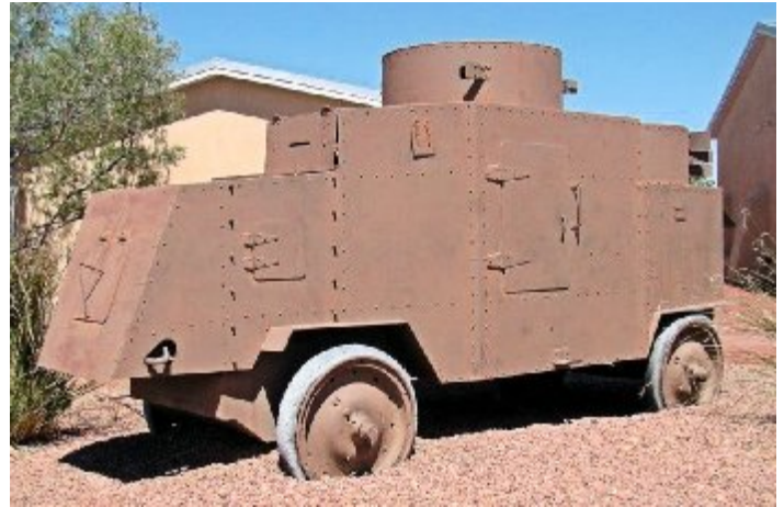
1915 Jeffry Quad truck armored with steel from the Bethlehem Corp. at the Rock Island Arsenal in Illinois. Had two manually operated turrets.
