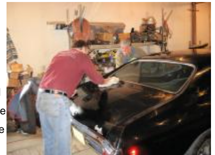
QUICK SHINE—Rick and John team up to put a quick coat of Carnuba Wax down on the cured paint
