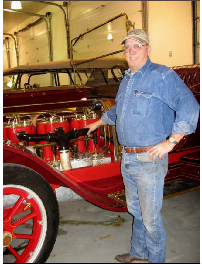
Willy is posing beside the 6-cylinder T-head inline engine of the 1912 Peerless Model 36.
