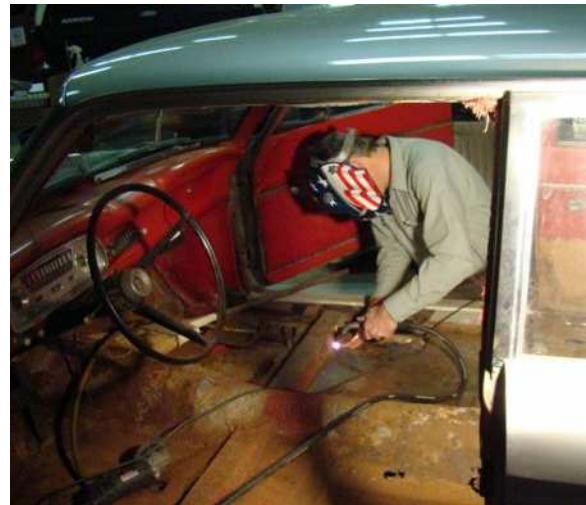
Charley Jurgens welds in a repair panel on the floorboard.
