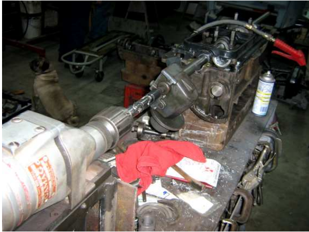
Honing the freshly poured babbitt.
