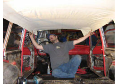
Above, John McFaul positions the new headliner. This became a rather tricky and labor intensive effort requiring windows to be removed.
