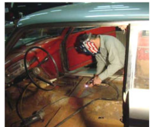
Above, Charley Jurgens welds in a repair panel on the floorboard.
