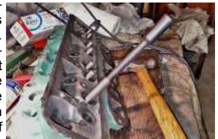
Driving in new valve guides with the proper driver tool.
