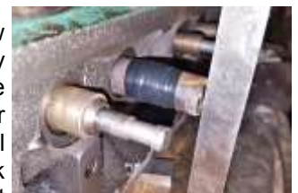
Made jigs or template gages to make sure valve guides were set at proper depth and to make sure valves were the proper length to the rocker arms after grinding the valve seats.
