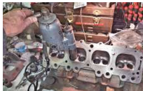
Using the Hall - Toledo Valve Seat Grinder to grind new seats, and trim them to proper width.
