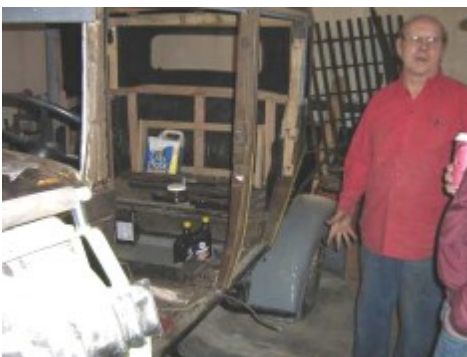
Don's LaSalle project required all new wood and rebuilding over every mechanical component, in addition to sheet metal work, painting, and a new interior.
