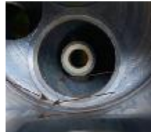
My cracked cylinder as posted on the Franklin Forum
